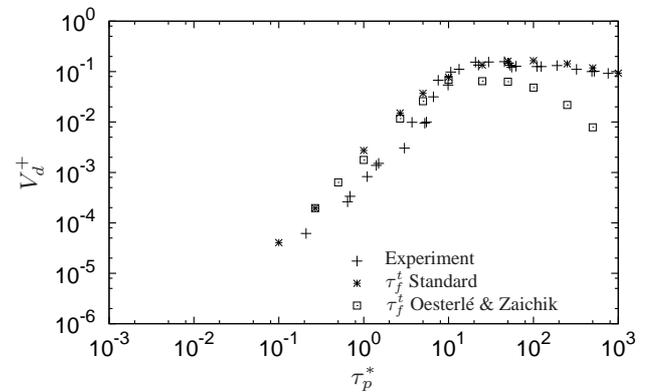
Figure 6: Deposition rate with respect to the Stokes number. Comparison between the experiments of Liu & Agarwal [10], the LBM prediction with  $\tau_f^t$  predicted by the standard model (20) and by the model proposed by Oesterlé & Zaichik (21) [14].
