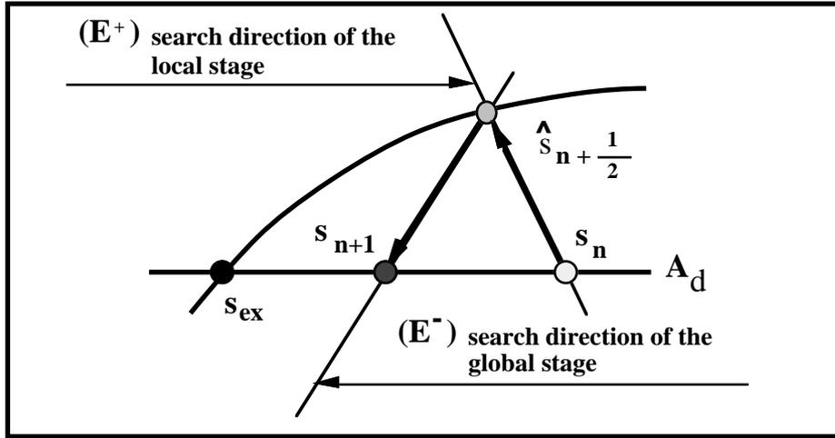
Figure 1: Iteration scheme
