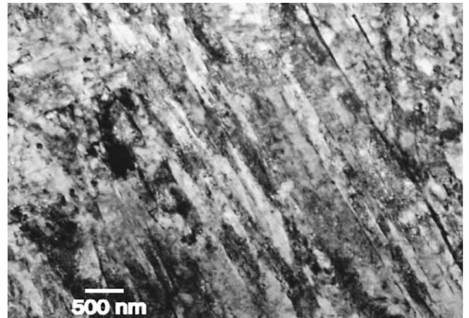
Fig. 2. Bright-field TEM image of the dislocation structure for the sample A4.
