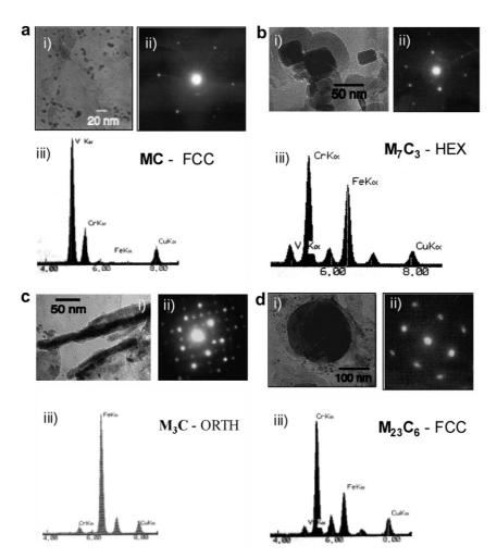
Fig. 4. Carbides morphology observed by TEM (bright field image, replica) (i), EDXS analysis (ii), electronic diffraction pattern (iii) for the four types of identified carbides: (a) MC, (b)  $M_7C_3$ , (c)  $M_3C$  and (d)  $M_{23}C_6$  in the reference grade.
