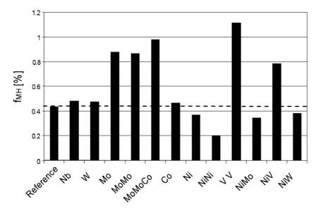
Fig. 6. Influence of alloying elements on the volume fraction of the first population calculated using the magnetic hole  $(f_{\rm MH})$  hypothesis.
