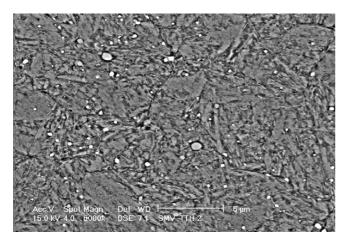
Fig. 5. SEM image showing numerous undissolved tungsten carbides (Nital etch) in the W grade.
