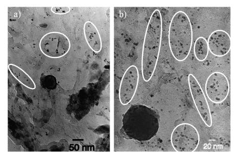
Fig. 12. Bright field TEM images showing the heterogeneous distribution of secondary vanadium carbides in the reference grade for a Nital etch time of (a) 5 s and (b) 15 s during the replica preparation. High number density zones are marked.
