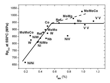
Fig. 9. Experimental yield strength measured at 550  $^{\circ}$ C as a function of the volume fraction of the first population estimated using the magnetic hole hypothesis (two tempering conditions for several grades).
