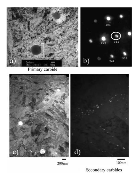
Fig. 7. (a) Bright field TEM image showing primary molybdenum carbides, (b) corresponding diffraction pattern, and (c) and (d) dark field TEM images showing the precipitation of both primary and secondary molybdenum carbides (MoMo grade), respectively.
