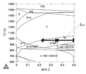
Fig. 2. Equilibrium phase diagram of the reference grade calculated by ThermoCalc<sup>®</sup> giving the proportion of carbides in the austenitic matrix.
