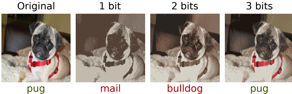
Figure 8: Example image, where a quantization (with dithering) using 3 bits leads to correct classification.
