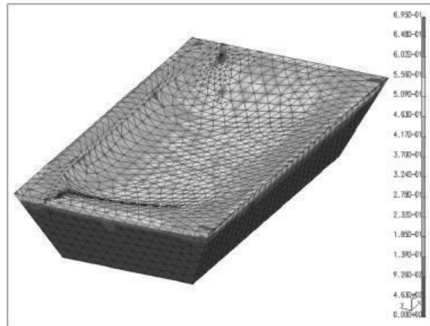
Fig. 9. Damage field generated by thermal gradients at a time of 300s after the tool extraction from the SPF press
