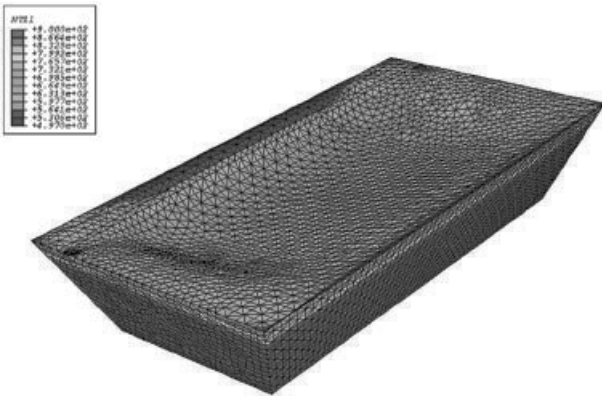
Fig. 5. Temperature field in the SPF tool at a time of 300s after the extraction from the press.
