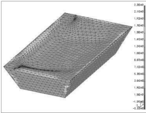
Fig. 10. Maximum principal stress field generated by thermal gradients at a time of 300s after the tool extraction from the SPF press
