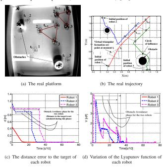
Fig. 7. Avoiding obstacles before joining the formation.
