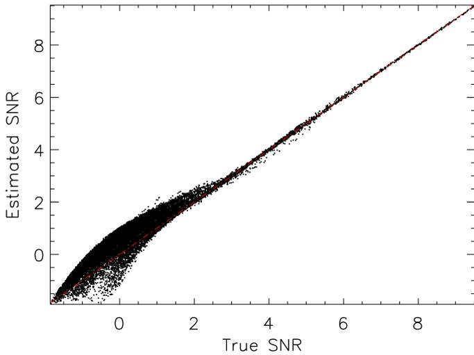
**Fig. 7.** Comparison of the estimated GGM filtered maps S/N as a function of the true S/N, using the RHAPSODY-G sub-sample. The estimated S/N is computed using the NIKA processed RHAPSODY-G sub-sample (Eq. (9)). The red dashed line represent the one to one correspondence. Each point corresponds to a pixel of the map.
