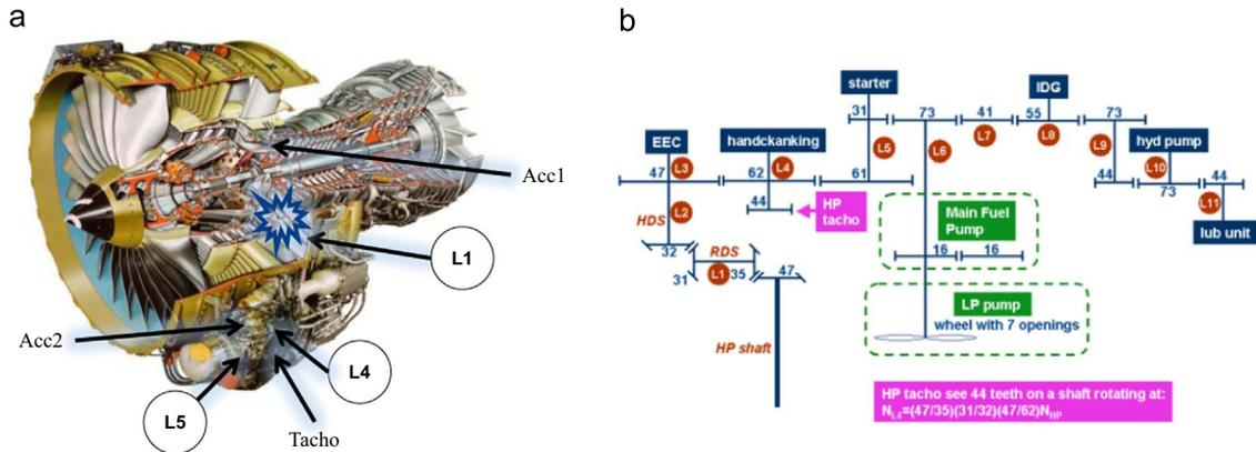
Fig. 14. (a) Sensor locations and (b) gearbox kinematics.
