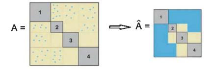
Fig. 1.4. Block structure preservation in the reduced-order matrix  $\hat{A}$
