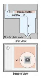
Fig. 1.12. A schematic overview of a single channel (courtesy of Herman Wijshoff)
