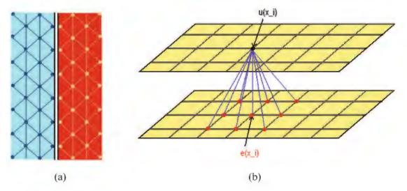
**Fig. 1.6.** Different types of strong coupling. (a) an interface coupling; (b) a strong coupling between different physical domains
