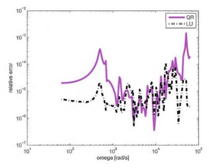
**Fig. 1.9.** Magnitude plots of the relative errors of the reduced-order frequency response functions based on different decompositions of the coupling blocks with respect to the reduced-order frequency response function based on the original input and output matrices
