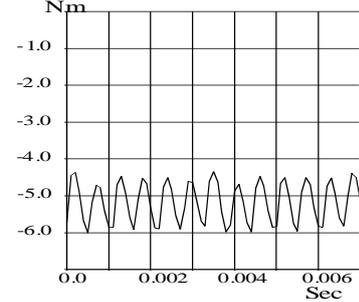
Fig.8 : Calculated torque at 3000 rpm.
