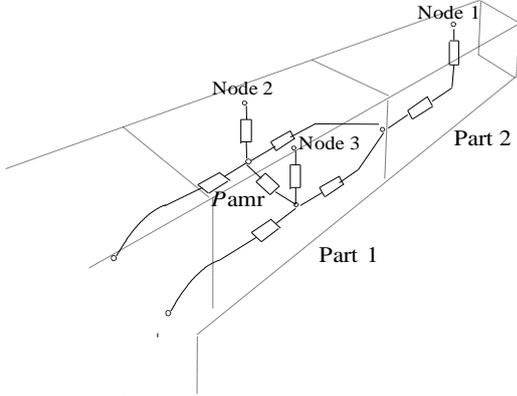
Fig.2: A claw-pole permeance network.
