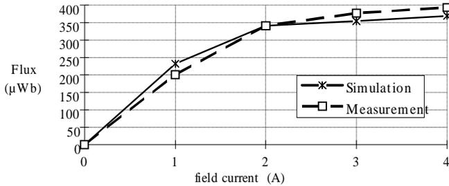
Fig.6: Stator flux phase at no-load versus rotor field current.
