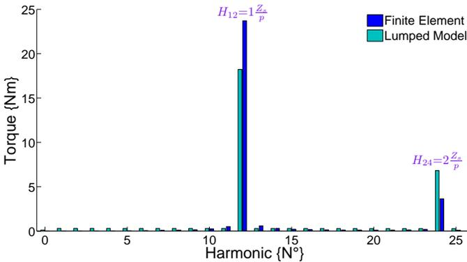
Fig. 16. Spectrum of analysis of cogging torque
