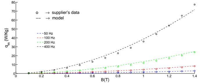
Fig. 8. Iron losses versus frequency and flux density
