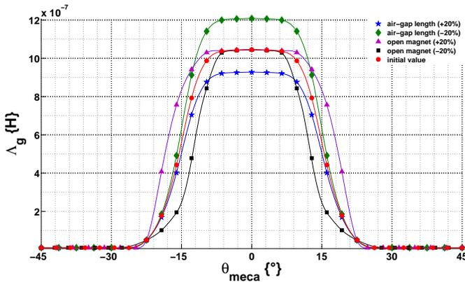
Fig. 7. Several evolution laws of the air-gap permeance
