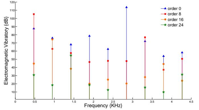
Fig. 11. Spectrum of electromagnetic vibrations for N=3555 rpm
