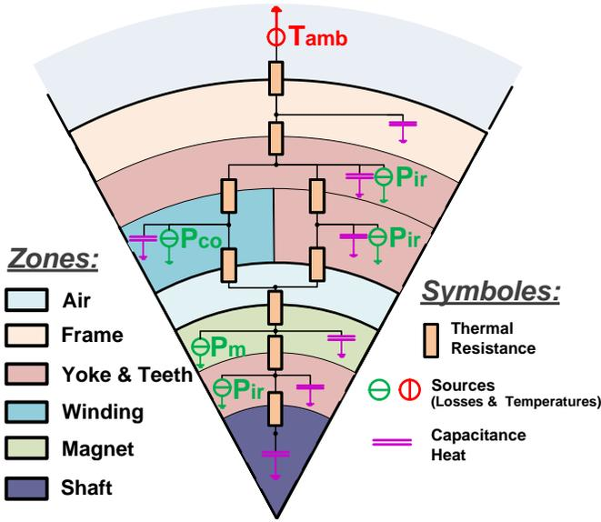
Fig. 9. Example of Nodal Network for PMSM.
