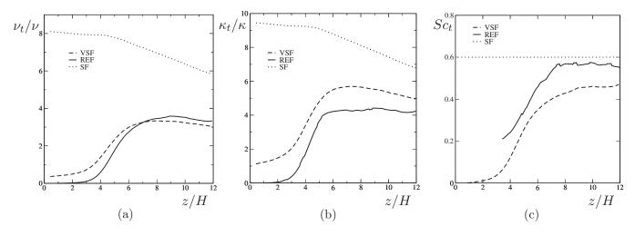
FIG. 2. Downstream evolution at y/H=0.5 of the (a) eddy-viscosity  $v_t$ , (b) eddy-diffusivity  $\kappa_t$ , and (c) SGS Schmidt number  $Sc_t$  in a priori tests on a plane jet for  $Re_H=3000$  and Sc=0.7. The reference values (REF) were obtained by box filtering the DNS, and using Eqs. (27), while results for the classical structure function model (SF), and viscous structure function model (VSF) were obtained with Eqs. (23)–(26), respectively.
