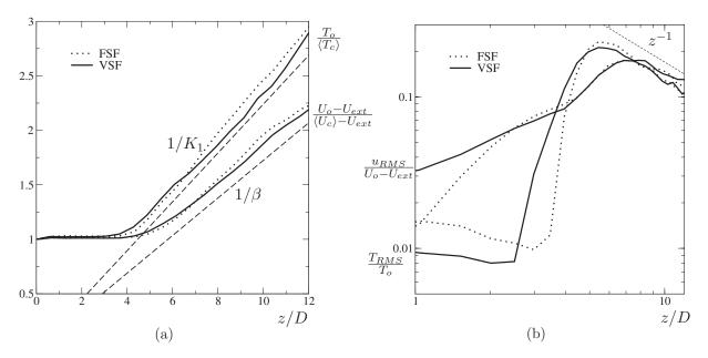
FIG. 3. Centerline evolution of the (a) mean velocity and passive scalar field and (b) RMS velocity and RMS passive scalar field for LES of spatially evolving round jets at  $Re_D = 25000$  and Sc = 0.2.
