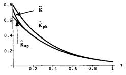
FIG. 7. The three memory functions for the bilaminated composite, n = 0.8.
