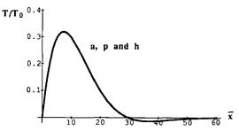
FIG. 8. Temperature profile in a semi-infinite bilaminated composite (n = 0.9) subjected to a cosinusoidal temperature variation at the origin, for the dimensionless pulsation  $\bar{\omega} = 0.02$ . h: homogenization; p: phenomenological approach; a: approximation.
