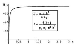
FIG. 4. Identification of the memory functions of the phenomenological and the homogenization approaches: the dimensionless heat transfer coefficient  $\bar{\omega}$  against the dimensionless time  $\tau$ .
