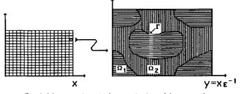
FIG. 1. Macroscopic and microscopic view of the composite.
