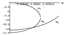
FIG. 5. Determination of the frequency for which the phenomenological and the homogenization approaches are equivalent. Bilaminated composite, n = 0.5.
