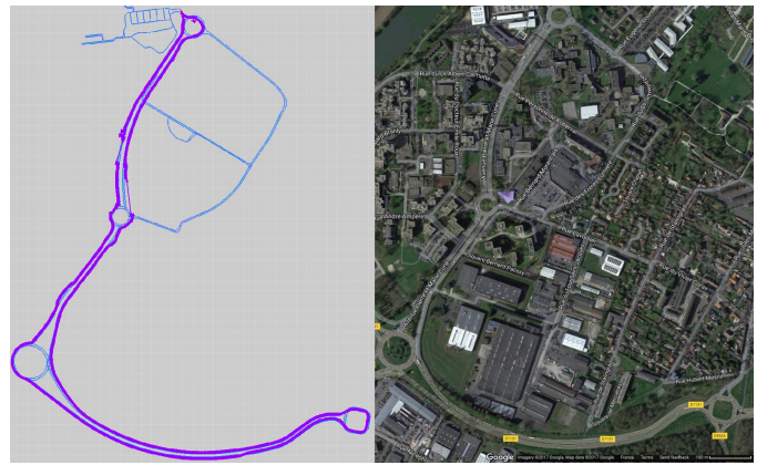
Figure 8. Left: test GNSS trace (in purple) over the lane map (in blue). This 4-km route is representative of a peri-urban trip (2-lane roadways, presence of buildings in certain areas as well as open-sky conditions in others). Large GNSS errors are clearly visible. Right: satellite view of the area (image from Google Maps).
