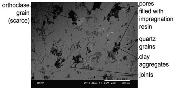
Figure 2: SEM image of a tight sandstone
