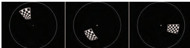
Fig. 12. Synthetic omnidirectional images used for the calibration
