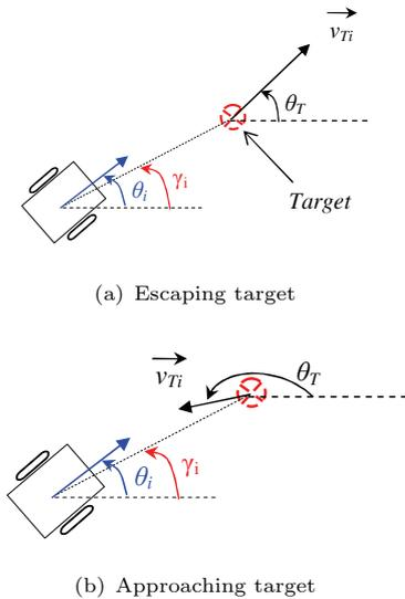
Figure 5: Escaping/Approaching target.
