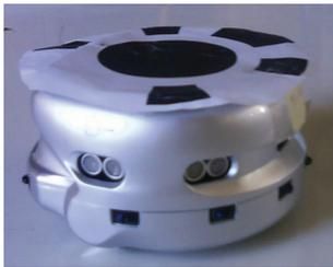
Figure 10: Khepera III mobile robot.
