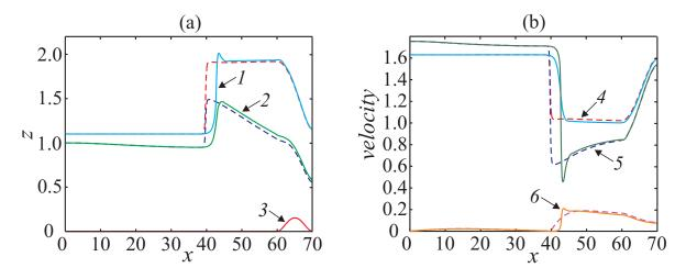
Figure 5: Quasi-steady turbulent bore: (a) shape of the bore (1 - free surface, 2 - internal boundaryz = h + b, 3 - bottom topography; (b) distribution of the velocities 4 - velocity U in the lower layer,  $5 - \text{velocity } \bar{u}$  in the upper layer, 6 - variable q. Solid curves refer to the solution of Eqs. (42), dashed curves correspond to the solution of the hydrostatic Eqs. (46).
