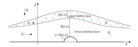
Figure 1: Two-layer stratified flow over topography.
