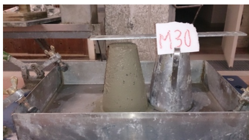
Slump at ( t=0 )
