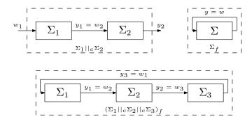
Fig. 1. Cascade, feedback compositions and an example of interconnection of systems
