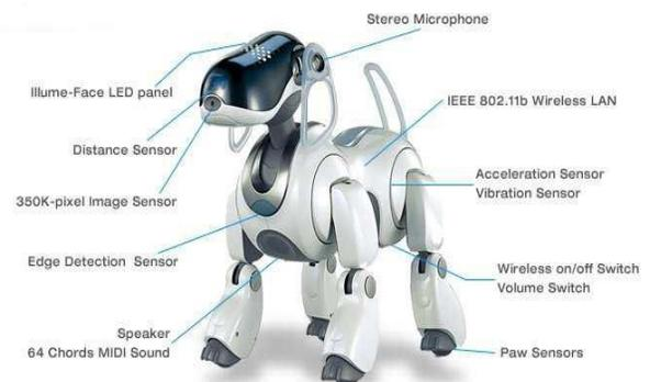
Fig. 13 The ERS-7 Sony Aibo Robot. (from <http://www.sony.net/Products/aibo/>)
