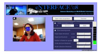
**Fig. 4.** Screenshot of the face analysis component, which runs on a PC and shows the analysis results through a MATLAB-based user interface It sends its results to the multimodal fusion module via TCP-IP.
