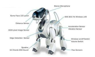
**Fig. 13** The ERS-7 Sony Aibo Robot. (from http://www.sony.net/Products/aibo/)
