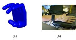
Fig. 12. (a) The 3D representation of the hand. (b) The CyberGlove<sup>®</sup>.
