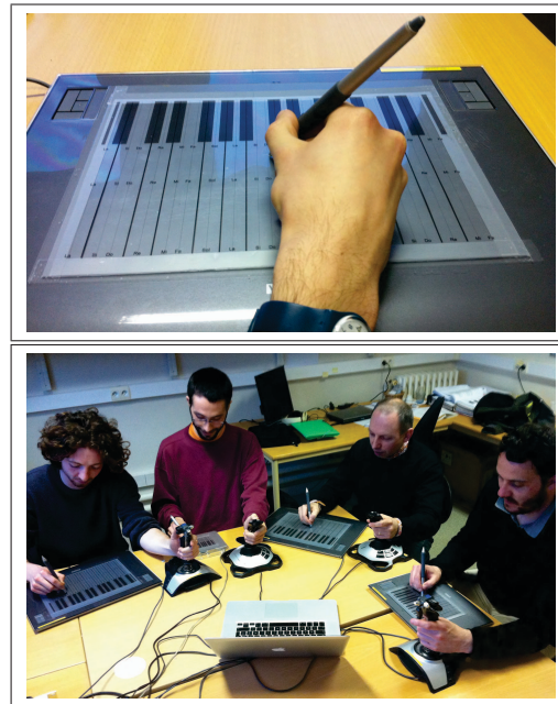
Figure 3: Keyboard for controlling the virtual singer (top). The Chorus digitalis performing (bottom).
