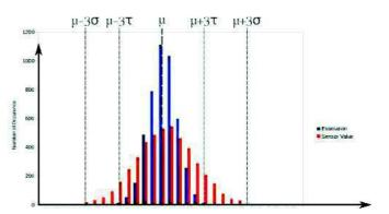
Figure 6. Gaussian distribution of a voltage sensor and the state estimation for a bus over multiple resolutions
