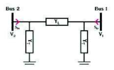
Figure 1. Example of  $\pi$ -line model
