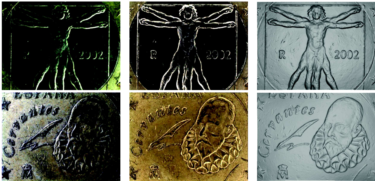
Figure 4. 3D-reconstructions of two metallic coins. From left to right: one of the m = 15 input images, estimated albedo and 3D-reconstruction. First row: Italian 1 euro coin. Second row: Spanish 50 cents coin.
