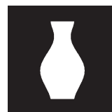
Fig. 8 Mask for the “Vase” dataset. The gradient values are only known on a non-rectangular part \Omega of the grid, represented by the white region. The FM and the CG-Poisson integrators can handle easily any form of domain \Omega . In contrast FFT, DCT, and Sylvester rely on a rectangular domain and therefore the values [p, q] := [0, 0] need to be fixed outside \Omega , in the black region.
