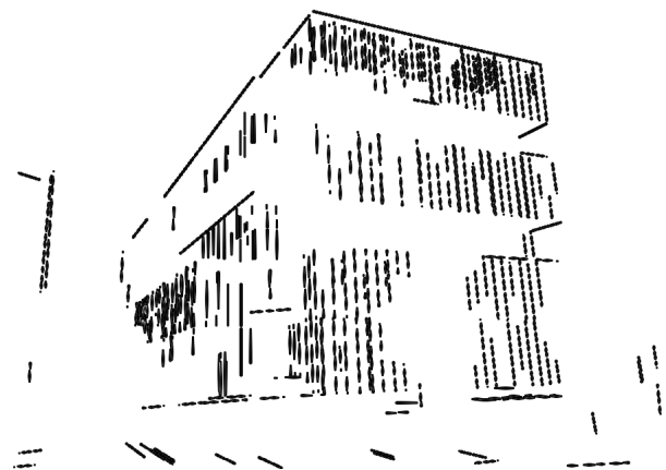
Figure 4. LSD segments detection.
