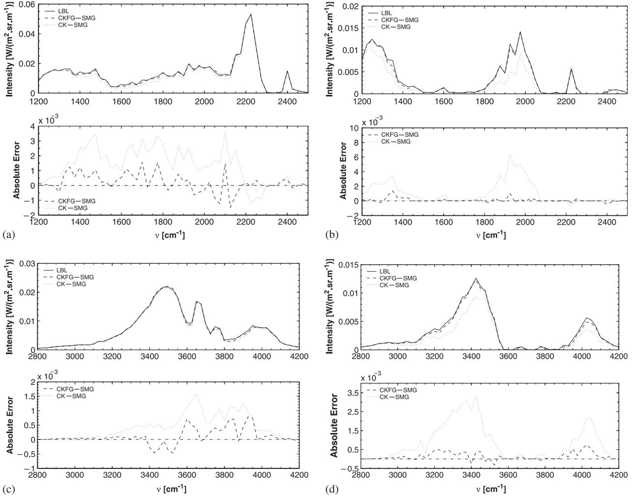
Fig. 4. Comparisons of narrow band radiative intensities spectra emitted from non-isothermal column and computed with LBL, CKFG-SMG and CK-SMG models: (a) 1200–2500  $\text{cm}^{-1}$  and  $\ell$  (300 K) = 0.2 m, (b) 1200–2500  $\text{cm}^{-1}$  and  $\ell$  (300 K) = 10 m, (c) 2800–4200  $\text{cm}^{-1}$  and  $\ell$  (300 K) = 0.2 m, (d) 2800–4200  $\text{cm}^{-1}$  and  $\ell$  (300 K) = 10 m.
