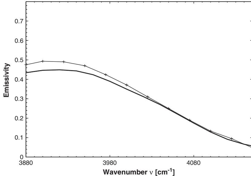
Fig. 2. H<sub>2</sub>O emissivity spectra between 3880 and 4180 cm<sup>-1</sup>: (- + -) experimental [37]; (—) calculated.  $T = 1450$  K,  $p = 1$  atm,  $x_{\text{H}_2\text{O}} = 0.1735$ ,  $\ell = 150$  cm.
