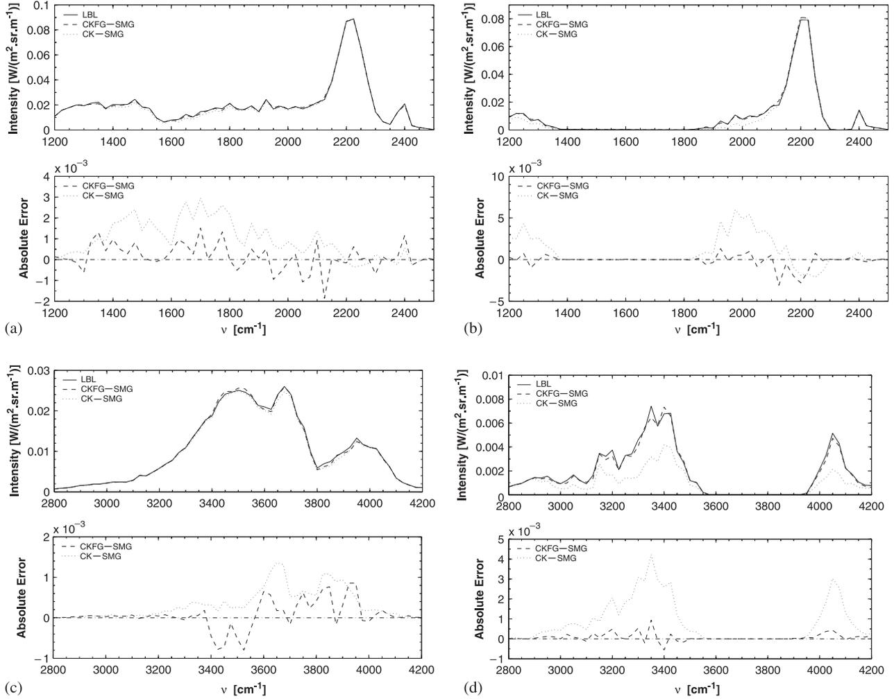
Fig. 5. Comparisons of narrow band radiative intensities spectra emitted from a non-homogeneous and non-isothermal column and computed with LBL, CKFG-SMG and CK-SMG models: (a) 1200–2500  $\text{cm}^{-1}$  and  $\ell$  (300 K) = 0.2 m, (b) 1200–2500  $\text{cm}^{-1}$  and  $\ell$  (300 K) = 200 m, (c) 2800–4200  $\text{cm}^{-1}$  and  $\ell$  (300 K) = 0.2 m, (d) 2800–4200  $\text{cm}^{-1}$  and  $\ell$  (300 K) = 200 m.
