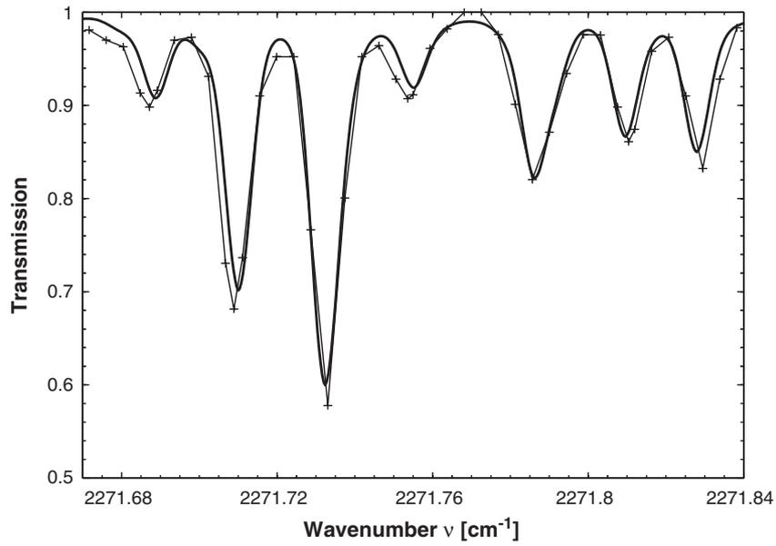
Fig. 1. CO<sub>2</sub> transmission spectra near 2271.75 cm<sup>-1</sup>: (- + -) experimental [36]; (—) calculated.  $T = 789$  K,  $p = 18$  mbar,  $x_{\text{CO}_2} = 1$ ,  $\ell = 11.48$  cm.
