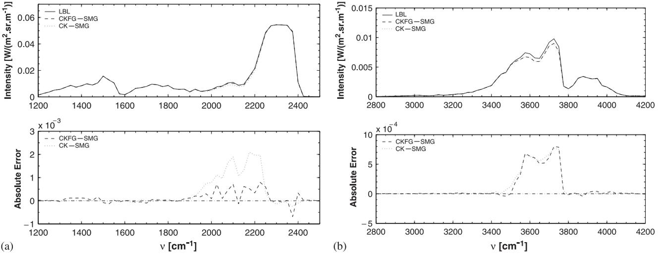
Fig. 3. Comparisons of narrow band radiative intensities spectra emitted from non-homogeneous column and computed with LBL, CKFG-SMG and CK-SMG models: (a) 1200–2500  $\text{cm}^{-1}$ , (b) 2800–4200  $\text{cm}^{-1}$  window.
