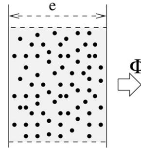
Fig. 1. Schematic representation of the total radiative flux  $\Phi$ , leaving the 1D layer composed of  $\text{H}_2\text{O}$ ,  $\text{CO}_2$  gases and a homogeneous monodispersion of spherical particles, both at thermal equilibrium.
