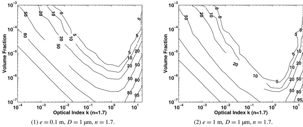
Fig. 6. Mappings of  $R_g$  [%] versus the volume fraction and the optical index  $k$ , for two values of the layer's thickness,  $e = 0.1$  m and  $e = 1$  m, containing particles with refractive index,  $n = 1.7$  ( $T = 2000$  K).
