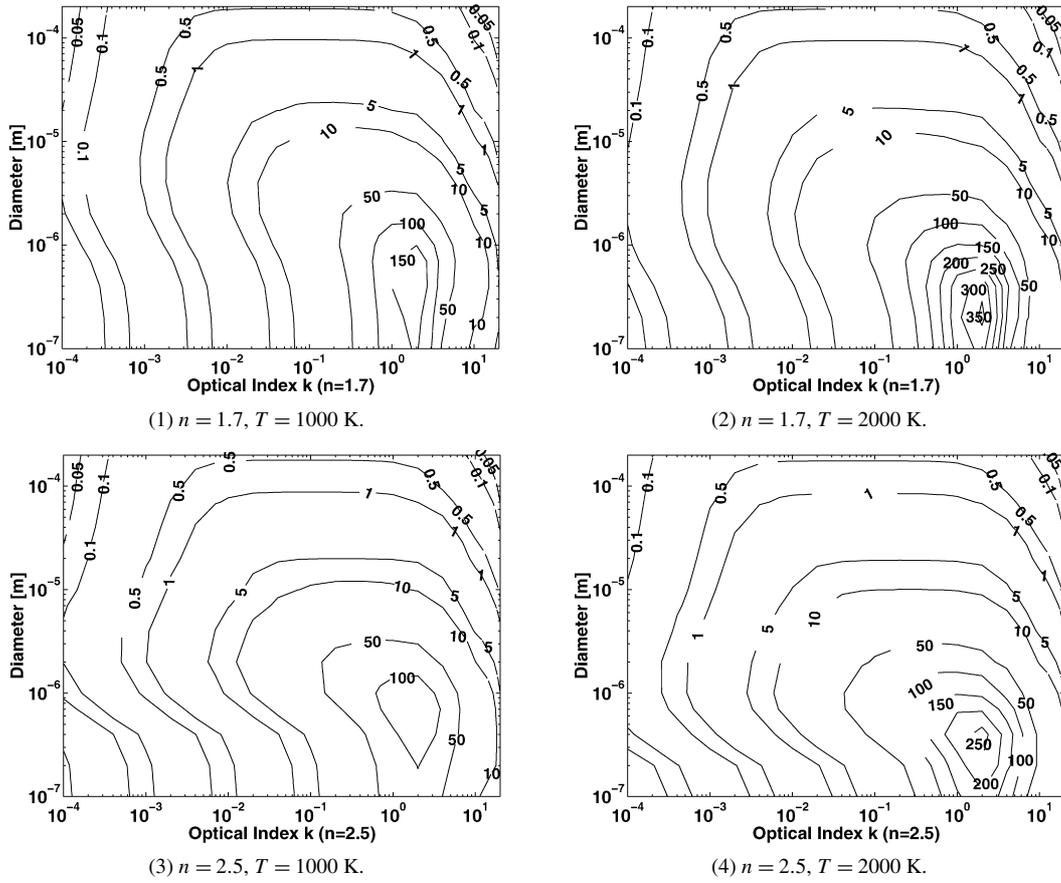
Fig. 2. Mappings of  $\frac{Q_p^*}{D} 10^{-4} [\text{m}^{-1}]$  versus the particle diameter and the optical index  $k$  ( $m = n - ik$ ), for two values of ( $n = 1.7, 2.5$ ), and for two values of the particle temperature, 1000 K and 2000 K.
