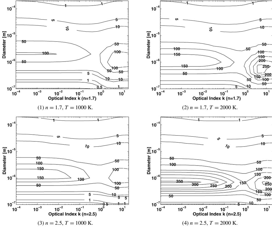
Fig. 3. Mappings of  $\frac{Q_s^*}{D} 10^{-4} [\text{m}^{-1}]$  versus the particle diameter and the optical index  $k$ , for two refractive indexes ( $n = 1.7, 2.5$ ), and for two values of the particle temperature.
