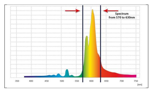
Figure 9: Spectrum of Indoorlux. Light is mostly emitted between 570nm and 630 nm.
