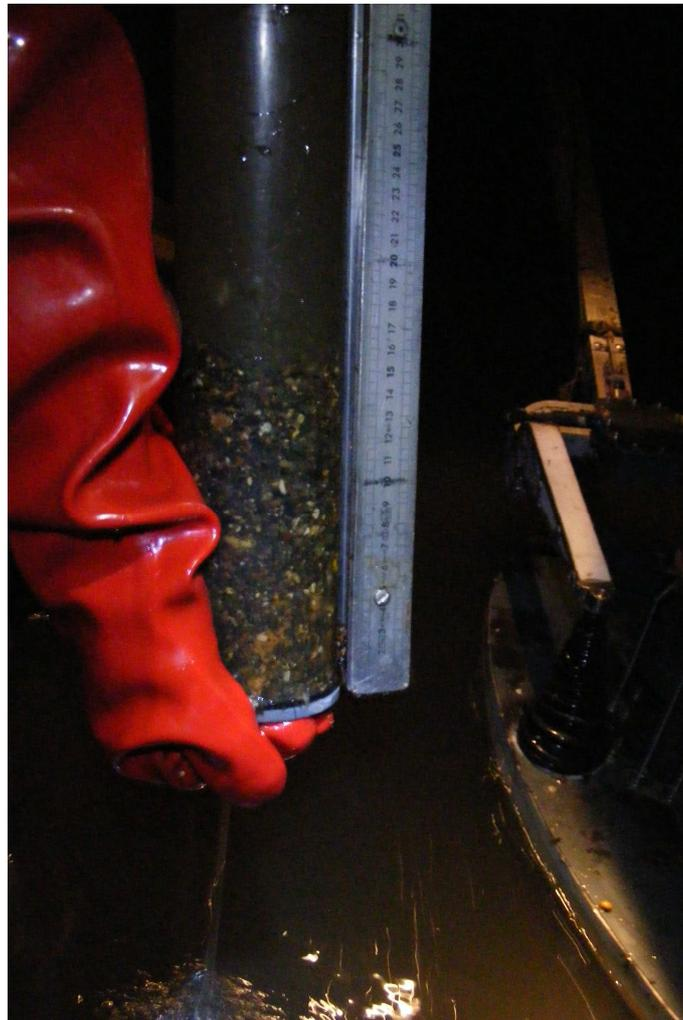
Figure 60 Sediment deposits surveyed with a clear Perspex cylinder of 7 cm of internal diameter.
