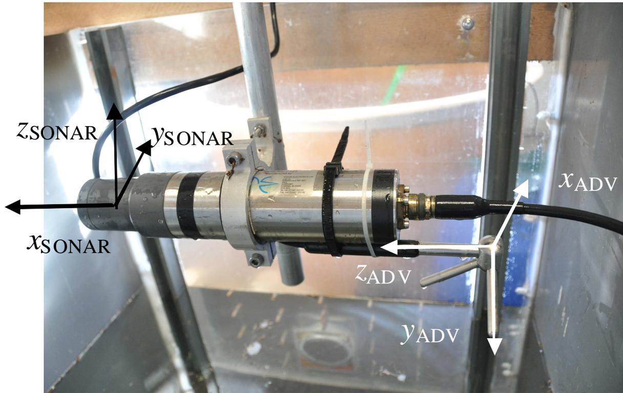
Figure 8 ADV and SONAR fastening (same as in-situ conditions)
