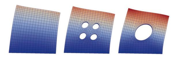
Figure 2. Deformed configuration for (from left to right)  $\Omega_0 \cup \Omega_1$ ,  $\Omega_0 \cup \Omega_2$  and  $\Omega_0 \cup \Omega_3$
