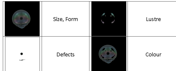
Fig. 5. Different segmented regions of a colour image of a Tahitian pearl and the quality parameters that are described in these regions.
