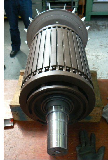
Fig. 11. New rotor of the industrial 250 kW motor.
