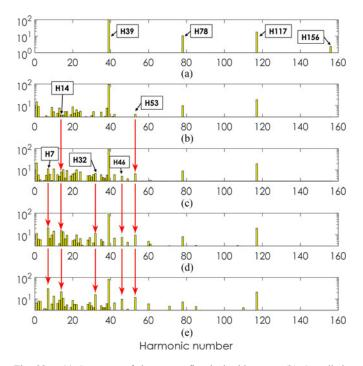
Fig. 32. (a) Spectrum of the sensor flu in healthy case. (b) One diode opened failure. (c) Two diodes opened failure. (d) Three diodes opened failure. (e) Four diodes opened failure. Let us note that the fundamental frequency (*H*1) corresponds to the mechanical one (25 Hz) and the frequency of the *H*39 is equal to  $f_e \times 39/p$  (975 Hz) where p is the number of pole pairs.
