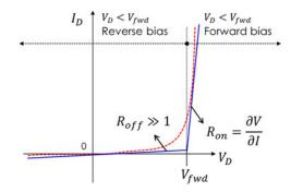
Fig. 12. Diode characteristics.
