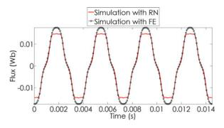
Fig. 14. Comparison with FE of tooth f ux,  $I_{exc} = 200$  A.
