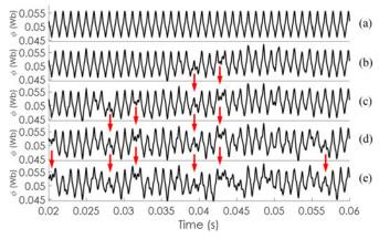
Fig. 31. Flux through sensor coil in healthy case (a), 1 diode opened failure (b), 2 diodes opened failure (c), 3 diodes opened failure (d), and 4 diodes opened failure (e). The time interval of 0.04 s corresponds to a mechanical period with frequency  $f_m = 25$  Hz.
