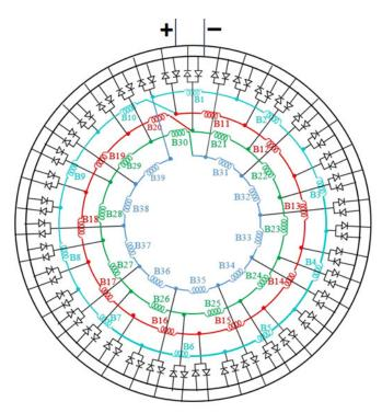
Fig. 3. Electrical diagram of the machine with the rectifie bridge.
