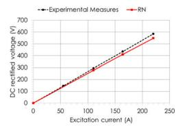
Fig. 19. Comparison of rectifie voltage versus excitation current curves in rated load tests.
