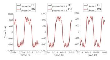
Fig. 23. Comparison of current in different phase coils in fault regime.
