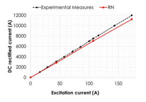
Fig. 20. Comparison of rectifie current versus excitation current curves in short-circuit tests.
