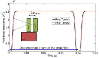
Fig. 9. Periodical evolution of the variable pole/tooth reluctance.
