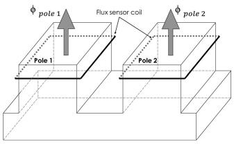
Fig. 30. Flux sensor coils placed on the poles and flu definitio associated.
