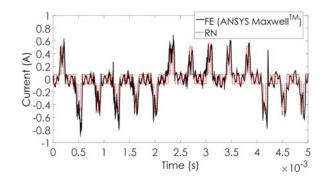
Fig. 16. Simulation of the current in the phase winding with finit element software (ANSYS Maxwell) and the RN model.
