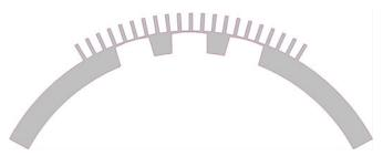
Fig. 5. Domain studied (shaded) to calculate the pole/tooth reluctance.
