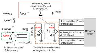
Fig. 10. Coupling circuit used to obtain the phase e.m.f. G1 = 1, G2 = -N, G3 = Rx, e.m.f.<sub>j</sub> =  $-Nd\varphi_{\text{total}}/dt$ .
