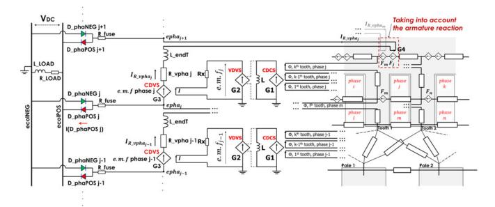
Fig. 11. Coupled circuit model.
