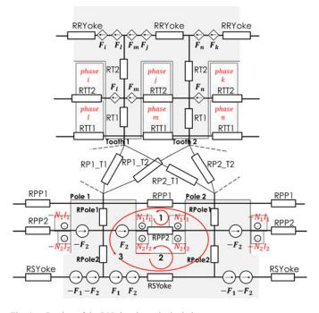
Fig. 4. Portion of the RN showing principal elements.
