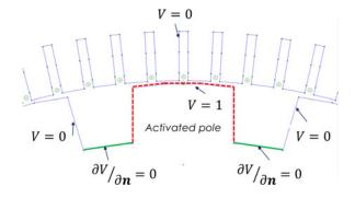
Fig. 6. Application of the boundary conditions.
