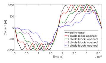
Fig. 29. Phase coil current wave form in healthy case and faulty states. The time interval corresponds to an electrical period ( $f_e = 275$  Hz).
