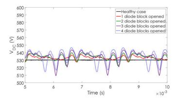
Fig. 28. Simulated rectifie output voltage in open diode fault regimes.
