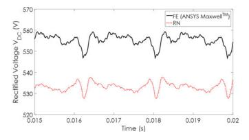
Fig. 22. Comparison of rectifie output voltage response in fault regime.
