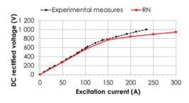
Fig. 15. Comparison of rectifie voltage measurements versus various de excitation currents.
