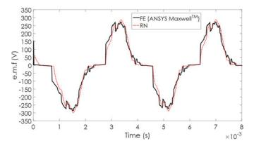
Fig. 17. Comparison of simulated electromotive forces.
