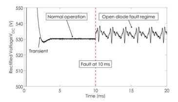
Fig. 21. Simulated rectifie voltage by RN model.
