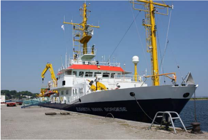
Fig. 6. RV EMB at the pier of the Naval Arsenal in Kiel, Germany. At this location it was equipped with a series of meteorological instruments and 4 corner reflectors mounted at the main mast, the bow and stern of the ship.
