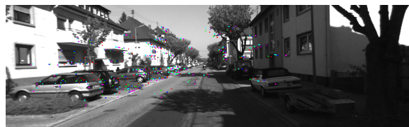
Fig. 4. Example of reprojection errors of the 3D points after BA, each color refers to the reprojection errors on a camera of the sliding window (5 cameras)
