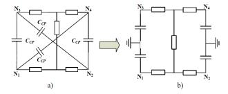
Figure 14: Our crosspoint models using a) real crosspoint capacitors and b) their equivalent grounded capacitors.
