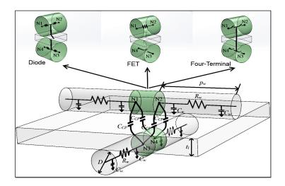
Figure 11: A nano-crossbar cell and its different forms for diode, FET, and 4-terminal switch based crosspoints.
