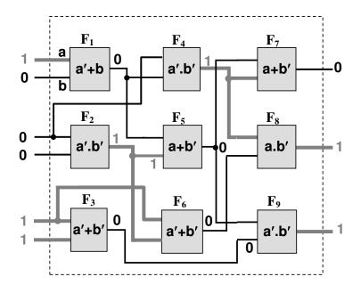
Figure 7: A logic network of single-term functions
