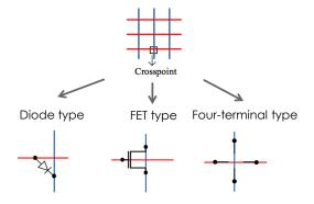
Figure 1: Different models of switching crossbars.
