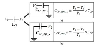
Figure 13:  $C_{CP}$  and its equivalent capacitors a)  $C_{CP-eqv-1}$  on  $V_1$  and b)  $C_{CP-eqv-2}$  on  $V_2$ .
