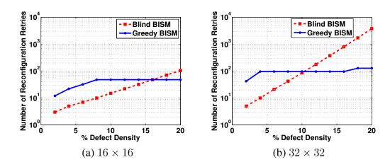
Figure 8: The number of configuration retries (a)  $16 \times 16$  crossbar (b)  $32 \times 32$  crossbar
