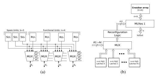
Figure 10: Reconfiguration technique for a crossbar array implemented with spare single function units. (a) shows the global architecture (for k=3 and n=4). (b) shows the connection with BIST unit.
