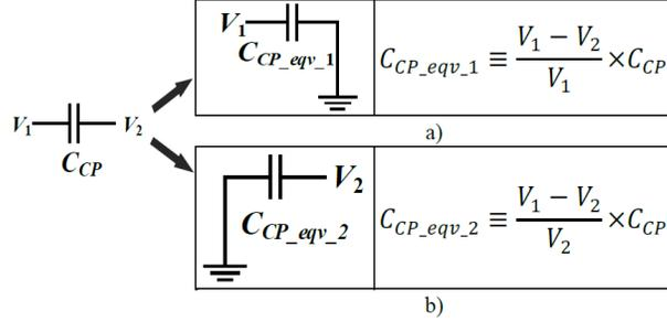
Figure 13:  $C_{CP}$  and its equivalent capacitors a)  $C_{CP-reqv-1}$  on  $V_1$  and b)  $C_{CP-reqv-2}$  on  $V_2$ .
