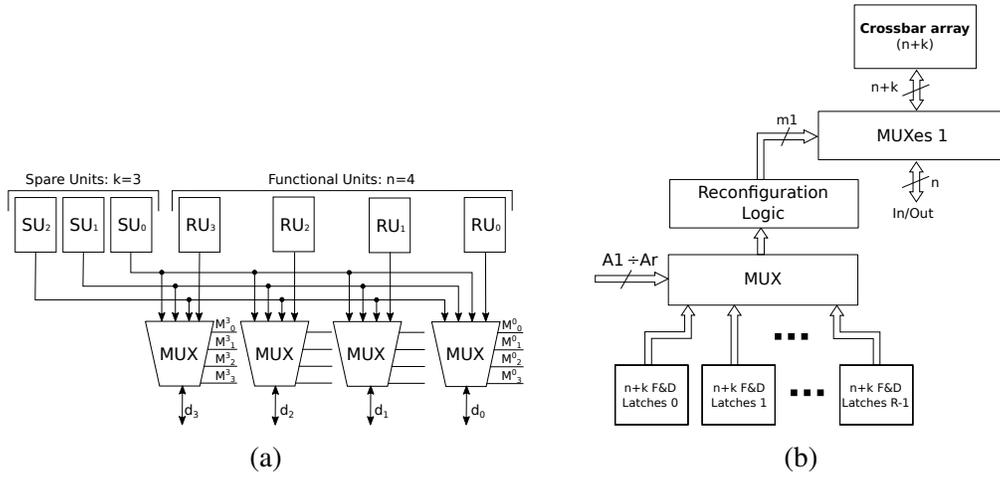
Figure 10: Reconfiguration technique for a crossbar array implemented with spare single function units. (a) shows the global architecture (for  $k = 3$  and  $n = 4$ ). (b) shows the connection with BIST unit.
