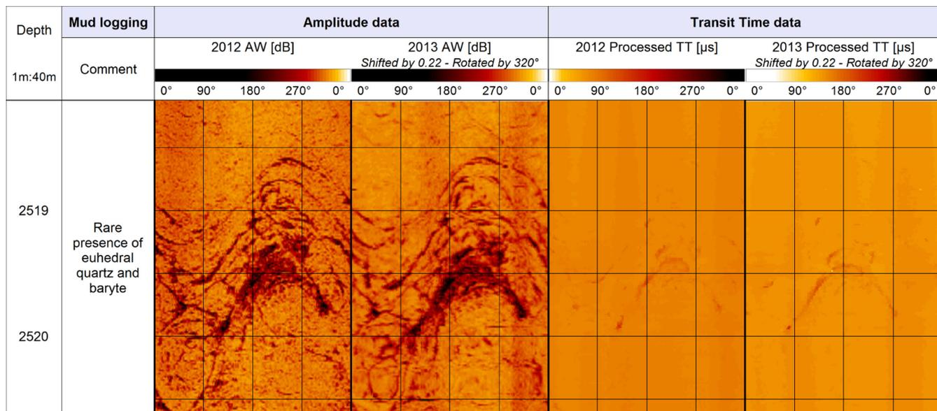
**Figure 6.** Comparison of acoustic image logs before and after the TCH stimulations showing a post-stimulation unmodified zone in the fresh granite. Amplitude data are expressed in dB, and transit time data in  $\mu$ s.
