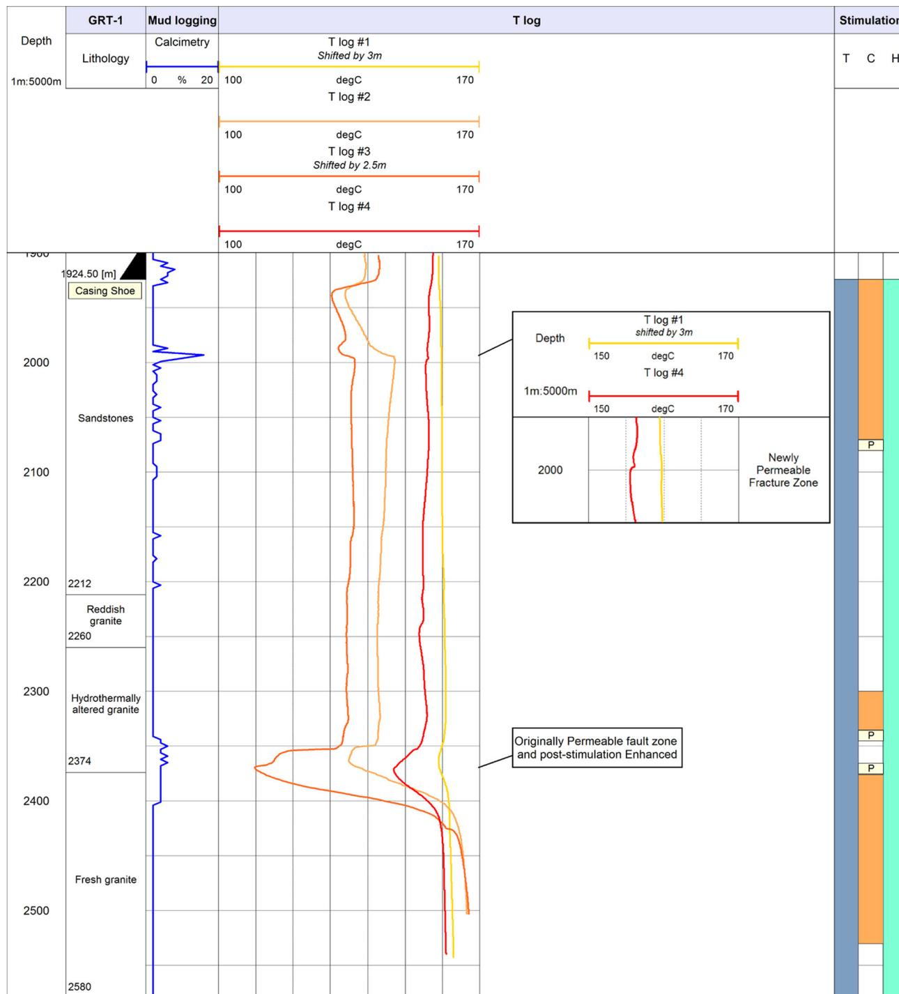
**Figure 3.** Composite log of well GRT-1. Calcimetry was measured by the mud-logging company. *T* logging operations were performed before the stimulations (*T* log #1), during the hydrochemical stimulation (*T* logs #2 and #3) and following the stimulations (*T* log #4). Stimulation zones are indicated.
