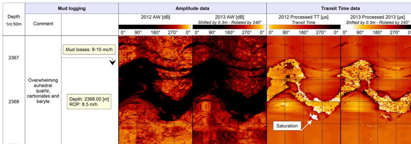
**Figure 12.** Comparison of acoustic image logs before and after the TCH stimulations showing an originally permeable and post-stimulation enhanced fault zone in the hydrothermally altered granite. Amplitude data are expressed in dB, and transit time data in  $\mu\text{s}$ .
