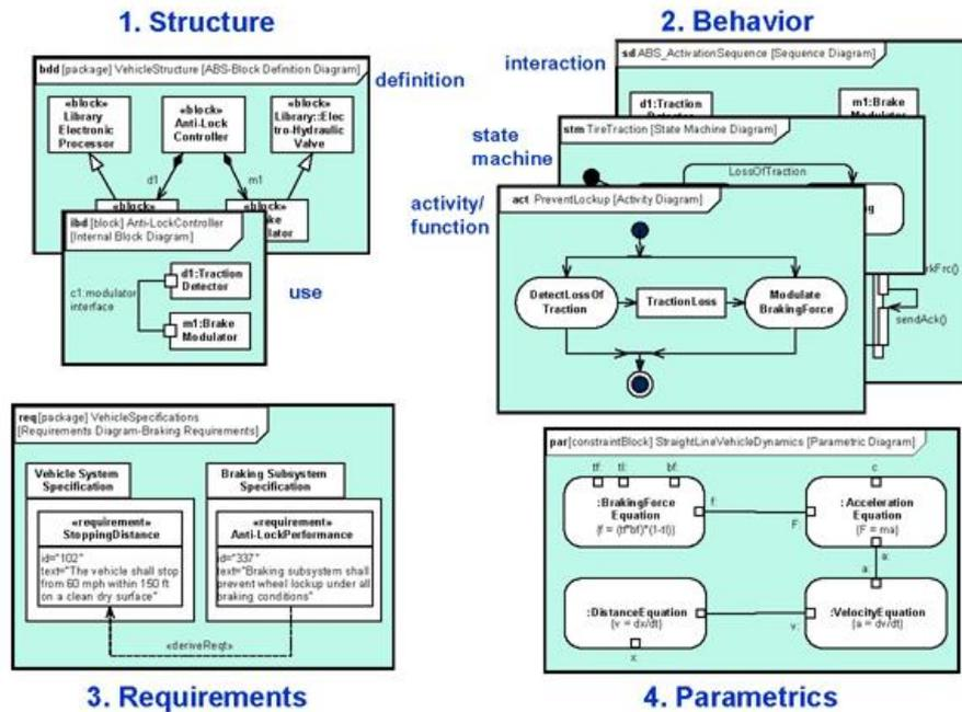
Figure 2 - The "Four Pillars" of SysML (OMG website)
