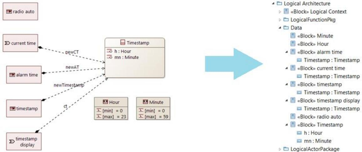
Figure 7 - Predefined Types transformation in SysML 1.4
