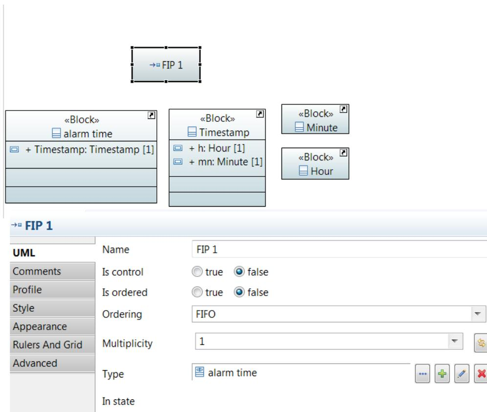
Figure 6 - Pin FIP1 typed with alarm clock
