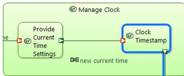
"Manage Clock" Capella Logique Function and its breakdown ("Provide Current Times Settings" and "Clock TimeStamp") are transformed to Activities + Call Behavior Actions (depicted in Papyrus Activity Diagram below). Functional Exchange "new current time" is mapped to Output pin and an Activity Parameter node+ Input pin and Activity Parameter node, interconnected with and Object Flow "new current time".
