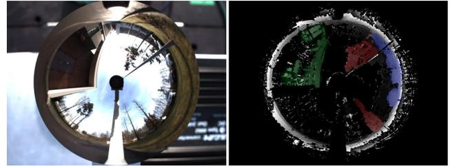
Fig. 10. Highlighting of the objects of the disparity map. By using the global method, the 3D reconstruction of the building (in green), trees (in red) and cars (in blue) is more complete.
