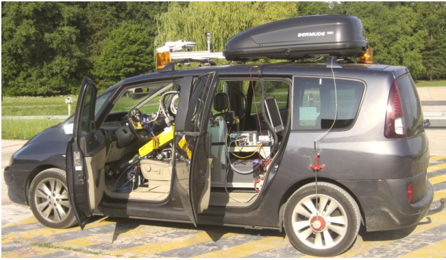
Fig. 3. Equipped car for autonomous driving
