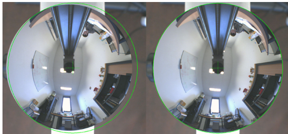
Fig. 3. Adjustment of the mirror position to respect the SVP constraint. The mirror border has to fit the estimation (green circle).
