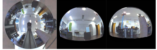
Fig. 9. An omnidirectional image and two views of its projection onto the unit sphere.
