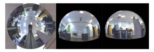
Fig. 9. An omnidirectional image and two views of its projection onto the unit sphere.
