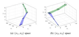
Fig. 6. Mode detection results of switched non-causal descriptor system
