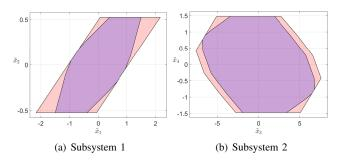
Fig. 1. The RPI and mRPI sets of equivalent causal descriptor subsystems: RPI sets (ultimate bounds) are plotted in purple region; mRPI sets are plotted in red region.
