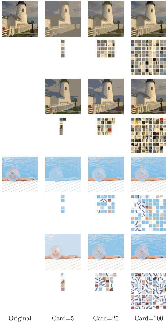
FIGURE 6: Image reconstruction: for each image, first two rows: original and reconstructions with uniformly sampled patches and below, the corresponding selected patches; second two rows: reconstructions with patches sampled according to a DPP and below, the corresponding selected patches.
