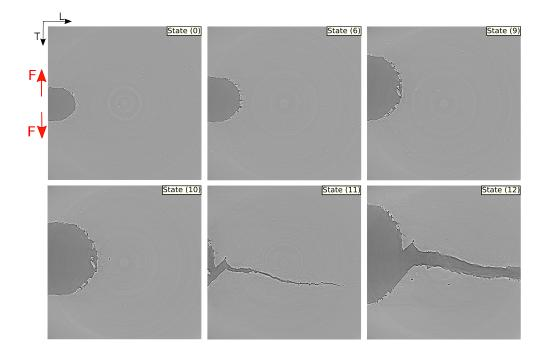
Figure 8: Mid-thickness sample section of the reconstructed volume for different loading steps indicated in every image
