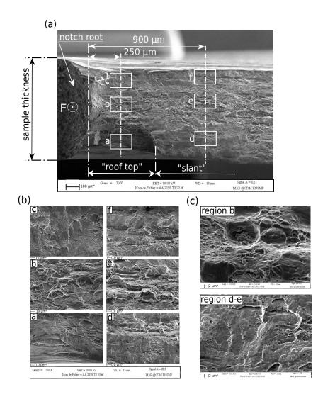
Figure 16: Scanning electron micrographs taken at one side of the broken CT-like specimen. (a) Magnification level  $\times 70$ , triangular zone at the notch root followed by slant surfaces. (b) Maginification level  $\times 700$ , magnified subsets **a-f** depicted in (a). (c) Maginification level  $\times 2000$ , zoomed details from subset **b** and from the zone between subsets **e** and **d**.
