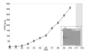
Figure 4: Notch Opening Displacement (NOD) for the step-wise loading procedure followed in this work; mid-thickness section showing the final crack propagated through the specimen ligament area for loading step (0)-(11)
