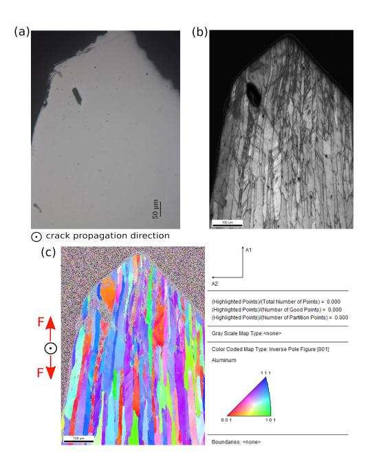
Figure 15: Electron backscattered diffraction taken at one side of the broken CT-like specimen on the section normal to the crack propagation direction. (a) View before electropolishing. (b) Grain texture revealing the transgranular nature of the inspected damage feature (denoted with red arrow in Figure 9 at State (11) and white arrow in Figure 14).
