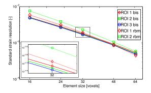
Figure 3: Standard von Mises strain resolution as a function of the element size used in the DVC procedure
