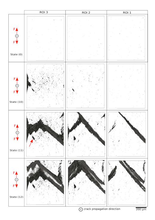
Figure 9: 3D visulaizations of segmented voids of ROIs 1, 2 and 3 for the undeformed configuration and last three loading steps
