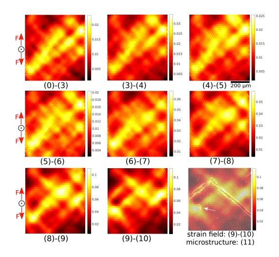
Figure 14: Incremental normal strain maps (in the loading direction) in ROI 2 (i.e., 460  $\mu$ m from the notch root) for different load steps and overlay of the last possible incremental strain field with the final crack path
