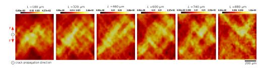
Figure 12: Sections normal to the crack propagation direction showing von Mises effective strain fields for loading step (0)-(3) for different distances from the notch root
