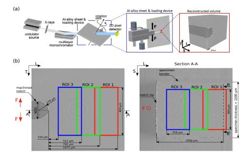
Figure 2: (a) Schematic view of the laminography setup with the loading device, CT-like sample and the scanned region (red zone). (b) 2D sections of laminography data indicating the positions of the Regions of the Interest (ROIs) examined in this work
