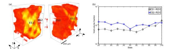
Figure 17: (a) Positions of the subsets depicted on the thresholded von Mises effective strain field. (b) Void growth over the loading history inside two subsets of ROI 1
