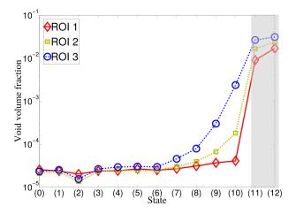
Figure 10: Void fraction development over the loading history for the three inspected ROIs (see Figure 2(b)). The shadow region denotes the final crack propagation through the ligament as shown in Figure 4
